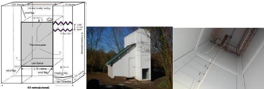
Figure 65: The experimental structure for measuring airflow in relation to the rate of partial pressure change as a small portion of air passed over the cooling coils and the contained water vapour condensed. The cooling coils seen from looking up the right-hand column. How much air was cooled per second depended on the rate of condensation and the resulting airflow. With no condensation there was no measurable airflow, even though the air at the cooling coils showed a temperature reduction of 10PC and a gain in density of 0.05 kilograms per m 3 – Peter Bunyard
